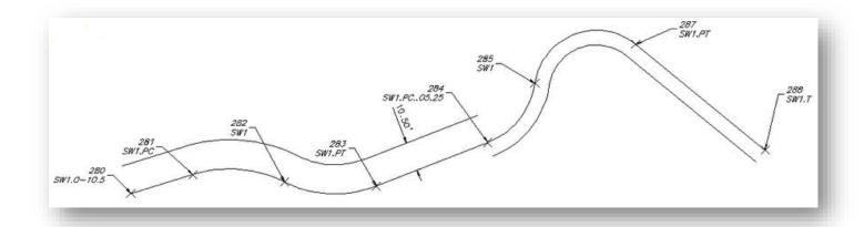
**Note:** There is not a transition from the first Offset code offset distance (-10.5) to the second Offset code offset distance (5.25); the first one stops, and the second one begins.
