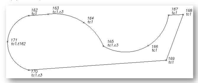
**Note:** Field crews do not have to add a description suffix at a point of reverse or compound curve, since the .C3 suffix code only reads the (3) consecutive points. Field crews can add a new C3 to start a new 3-Point Curve. PConnect checks for direction changes between segments and automatically determines the presence of a PRC or PCC, so there is no need to identify the PRC or PCC when using the C3 suffix code. See points162 - 171 above.
