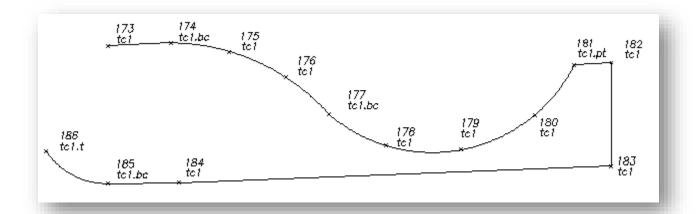
**Note:** If only two points are encountered after the Best Fit Curve (.BC) code, and the bearings created between the first two points and the second two points differ by less than five (5) degrees, the Begin Curve (.PC) calculation method is used to create a reverse curve. If the Best Fit Curve method was used, the curved segments would appear almost like two straight segments.
