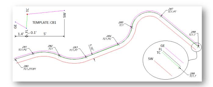
The third offset polyline, GE1 (magenta line), is drawn at 1.5 (0.1 + 1.4) units to the left of the original path of the collected points, starting at point 280 and ending at point 288, creating <u>curves</u> and <u>lines</u> per the encountered <u>suffix codes</u>.
