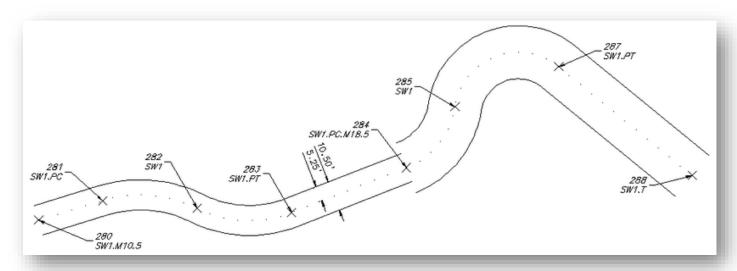
**Note:** There is not a transition from the first Middle code offset distance (10.5) to the second Middle code offset distance (18.5); the first one stops, and the second one begins.
