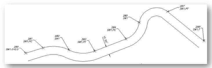
Note: The offset polylines will create a fillet with a zero (0) distance if the offset is larger than a calculated curve radius.
