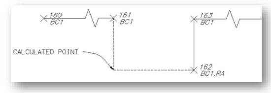
**Note:** This suffix code requires at least two prior points to calculate the starting angle and at least one point to calculate the ending angle. If there is no solution, parallel lines, or the calculated point is too far away, a straight line is drawn between the two points and a warning message is displayed at the end.
