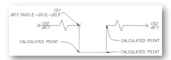
**Note:** The code assumes the previous segment was a straight segment, and this suffix code is ignored if in the middle of any of the curve suffix codes. This code can be combined with a termination code (.T, .CS, or .CC).
