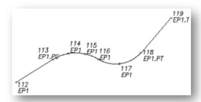
**Note:** Field crews do not have to add a description suffix at a point of reverse or compound curve. As long as there is not a straight segment, do not add the End Curve (.PT) code, and the command will draw the reverse or compound curve segments. PConnect checks for direction changes between segments and automatically determines the presence of a PRC or PCC, therefore, there is no need to identify the PRC or PCC with a PT/PC.
